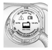
The engine coolant surge tank is located toward the rear of the engine compartment on the driver side of the vehicle. See *Engine Compartment Overview on page 10-10* for more information on location.
